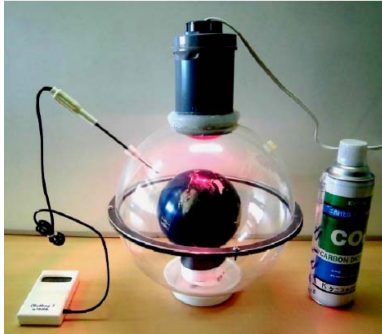
Photo 1. Real view of the model instrument for experiment of global warming.
