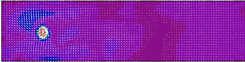
**Figure 5.** Flow field of free surface in tundish.
