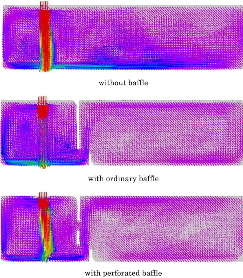
**Figure 7.** Comparison of flow field in tundish with different schemes.
