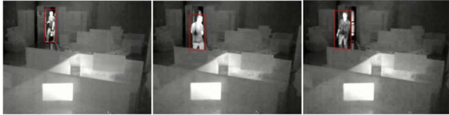
(a) Infrared video image mean-shift filter tracking results
