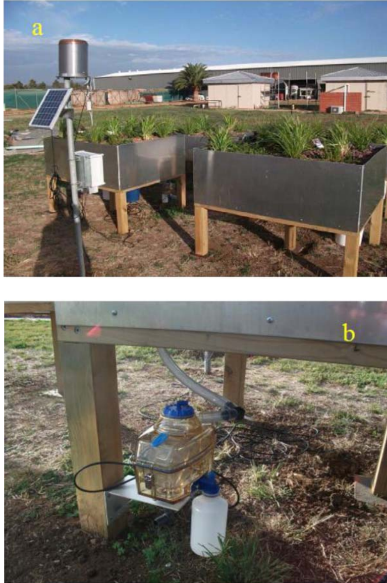
Figure 3. Green roof beds: (a) rain gauge and data logger; (b) outflow runoff tipping counter.
